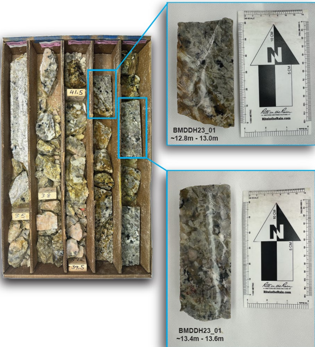
Figure 2: Black Mountain pegmatite intersection in BMDH23_01 from 10.5m (34.5ft.) to 13.7m (45ft.) showing some of the spodumene mineralization (See Chariot's ASX Announcement dated 2 February 2024)
