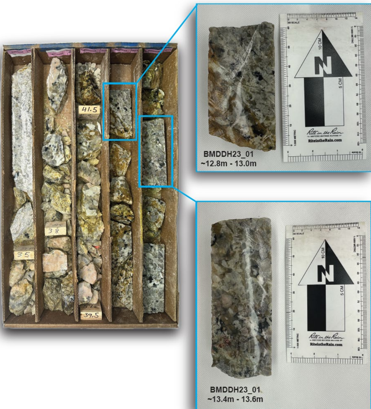
Figure 2: Pegmatite intersection in BMDH23_01 from 10.5m (34.5ft.) to 13.7m (45ft.) showing some of the spodumene mineralisation.
