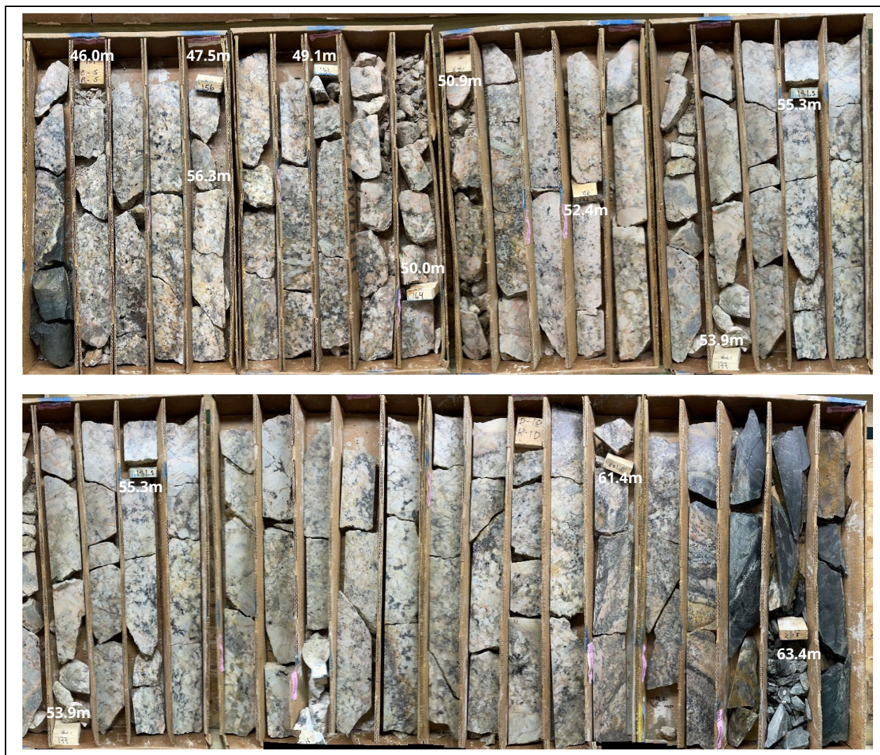
Figure 6: Pegmatite intersection in BMDDH23_03 from 45.3m (161ft.) to 63.4m (208ft.).
