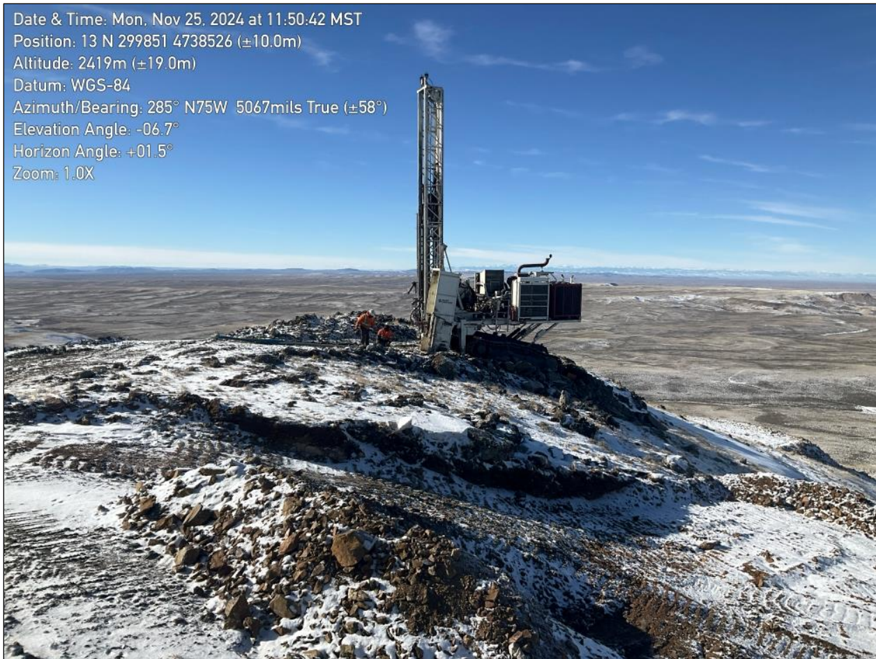
Figure 1: Boart Longyear MPD 1500 Reverse Circulation Drill Rig at Black Mountain
